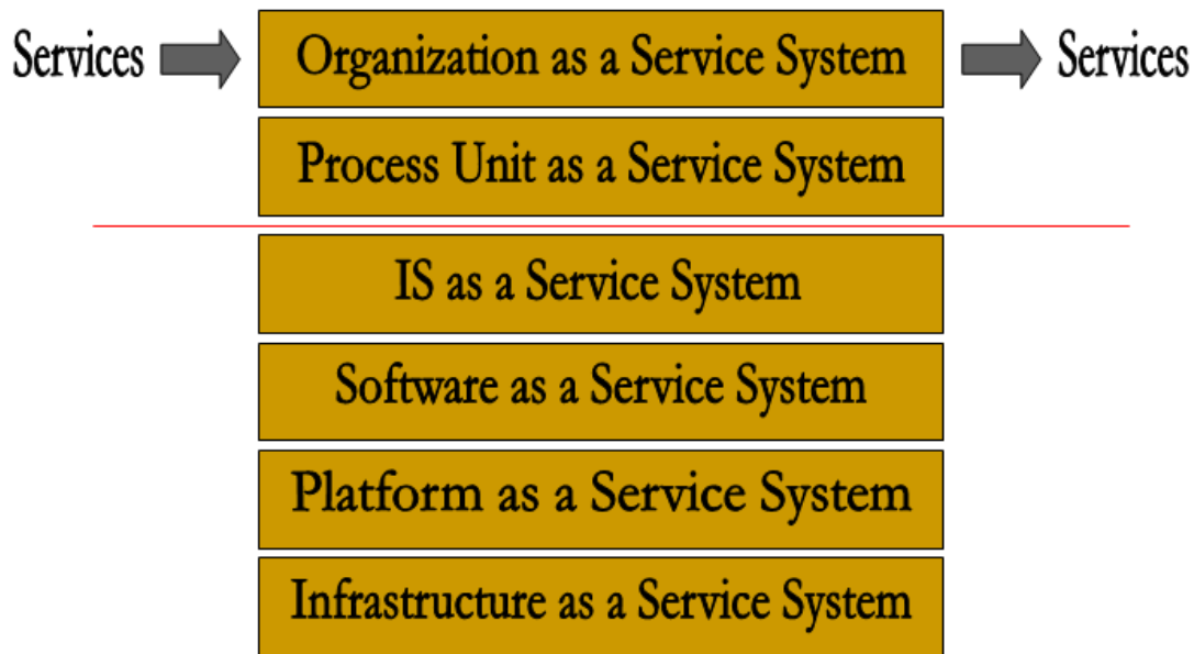
Figure 6: Organization as a service system and the layer structure of an organization. Systems in the lower layers provide services to the higher layers. Service units could provide services to other service units within the same layer.
