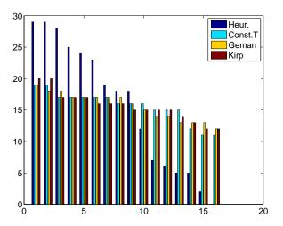
Fig. 12. Number of readers assigned to different time slots for nonprogressive algorithms. The total number of slots is 16.
