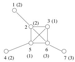
Fig. 2. A simple reader network. The numbers inside the parenthesis correspond to the time slots being assigned.
