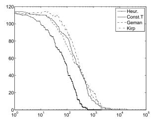
Fig. 11. Number of reader collision pairs against the number of iterations. The total number of slots is 16.
