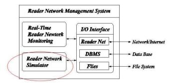
Fig. 18. Three modules in the reader network management system.
