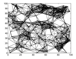
Fig. 10. 250 readers in random locations within an area of  $100m \times 100m$ . Readers at the end of an edge are neighbors.
