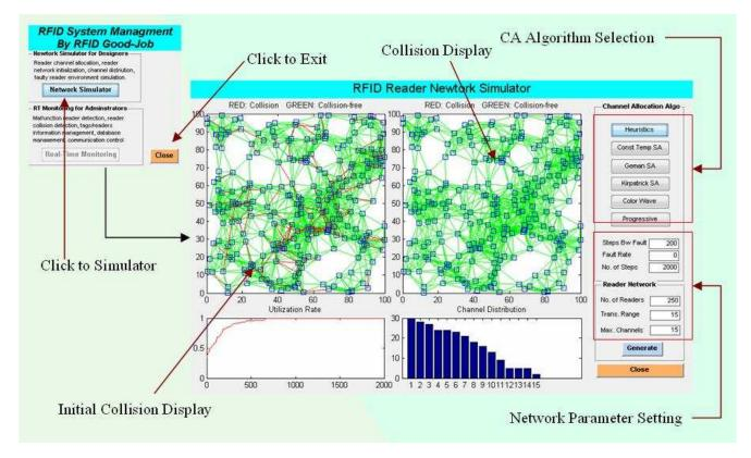
Fig. 16. Simulator for reader network management.
