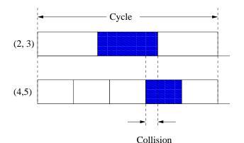
Fig. 21. Reader collision due to different values of local maximum color.
