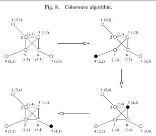
Fig. 9. Illustrative example for the Colorwave algorithm.
