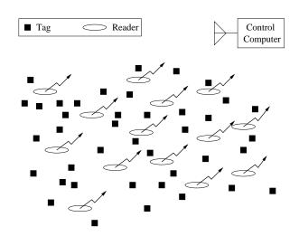
Fig. 1. An RFID reader network, with readers communicating to the control computer via a wireless LAN.
